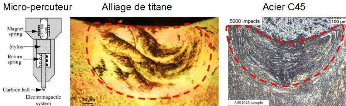
FIGURE 4. Left : sketch of the micro-impact tester. Right : cross-section of the indent zone after 5000 impacts on a titanium alloy (Sekkal *et al.* [2]) and on an AISI1045 steel.
