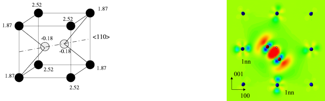
Figure 5: typical results obtained using DFT calculations \langle 110 \rangle SIA configuration and the local magnetic moments carried by the atoms in bcc Fe. Carbon-carbon covalent bond interaction (red atoms) within a single vacancy (white square)
