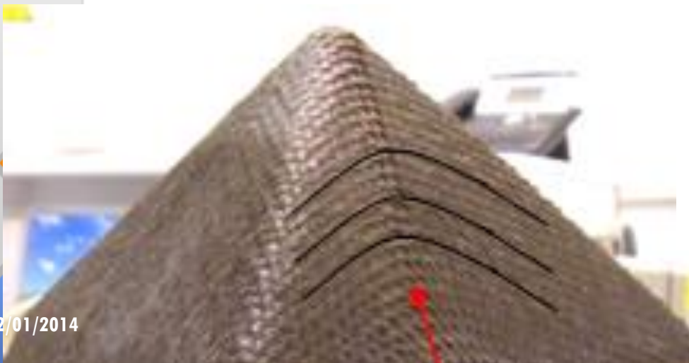
Tow buckles ( out of plane bending of tows ) on a face
