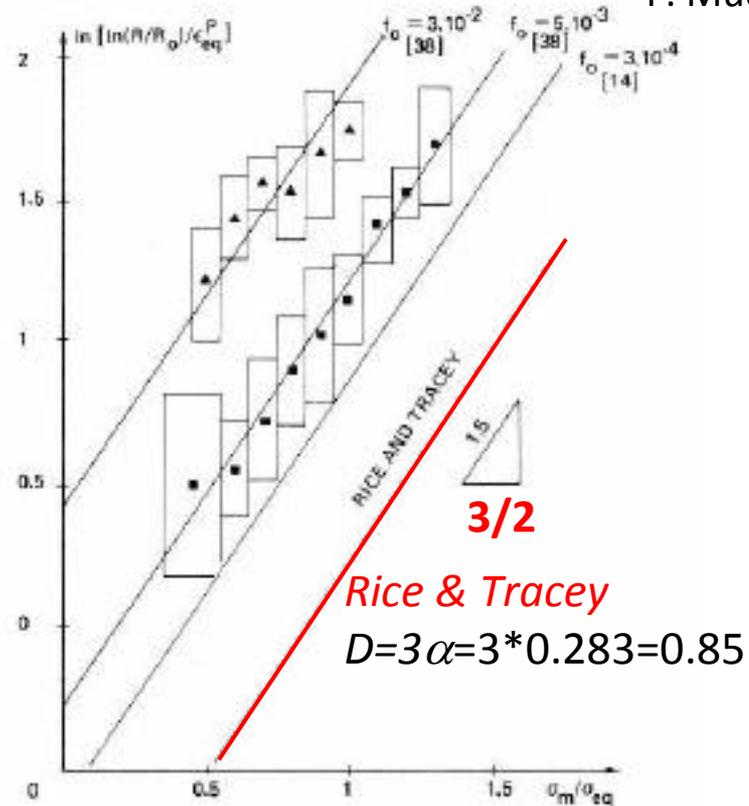
Fig. 3. Verification of the relation expressing the growth of cavities in a low alloy forged steel [14] and forged sintered steels [38].
