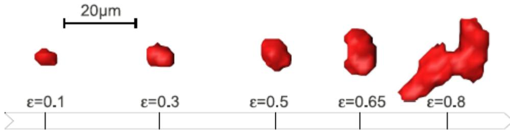
Figure 3.6: 3D visualization of the same cavity at different steps of deformation in the DP11 sample.
