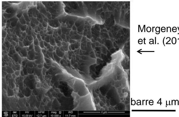
Fig. 14. Fractography taken in the slant fracture region showing nanometric dimples (at  $\sim 1$  mm from the notch of a different specimen).
