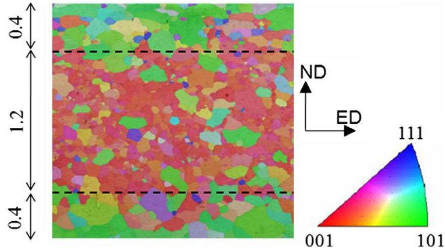
Extrusion AA6260-T6, pôles {111}, EBSD a (2 mm) et b (couche centrale 1.2 mm)
