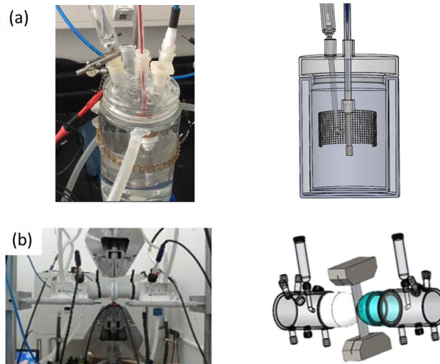
Figure 1 : Photo and scheme of (a) electrochemical charging of cylindrical specimens and (b) permeation assembly on the tensile machine.
