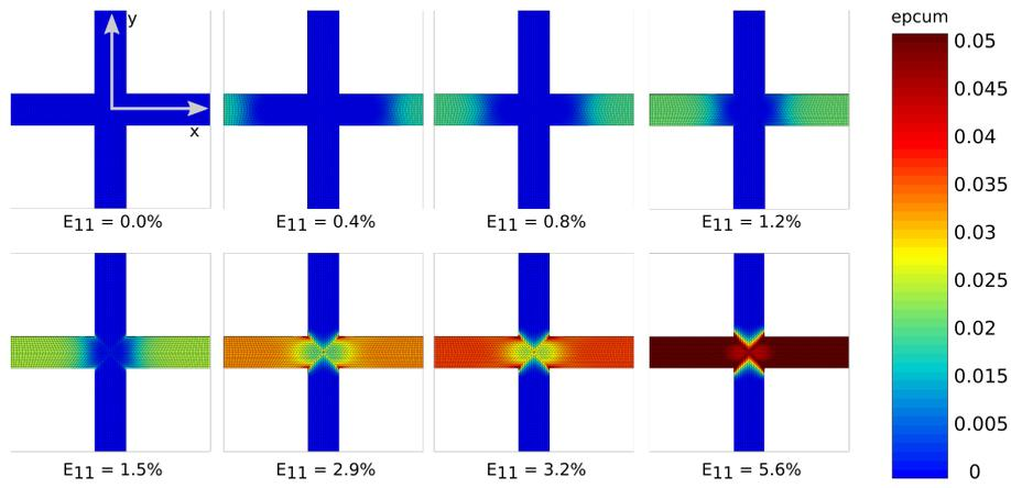
FIGURE 6 – Diamond lattice rotate from an angle of  $0^\circ$  and loaded in X direction
