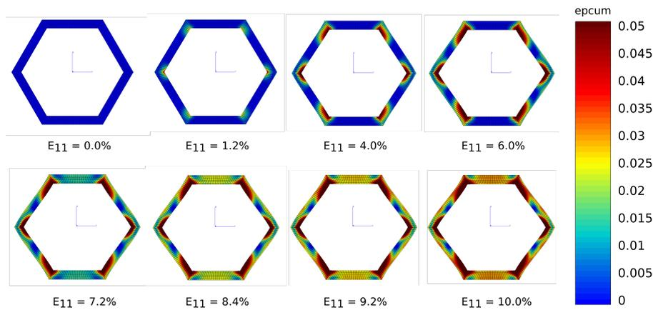
FIGURE 8 – Hexagonal lattice rotate from an angle of 0 degree and loaded in X direction
