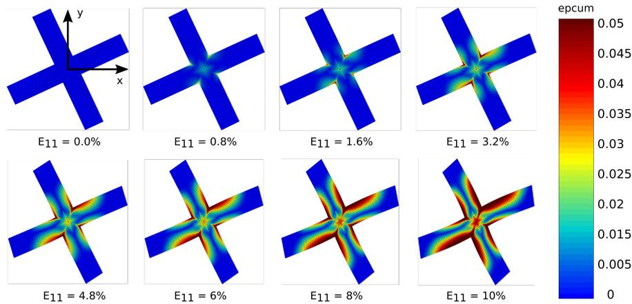
FIGURE 5 – Diamond lattice rotate from an angle of  $25^\circ$  and loaded in X direction
