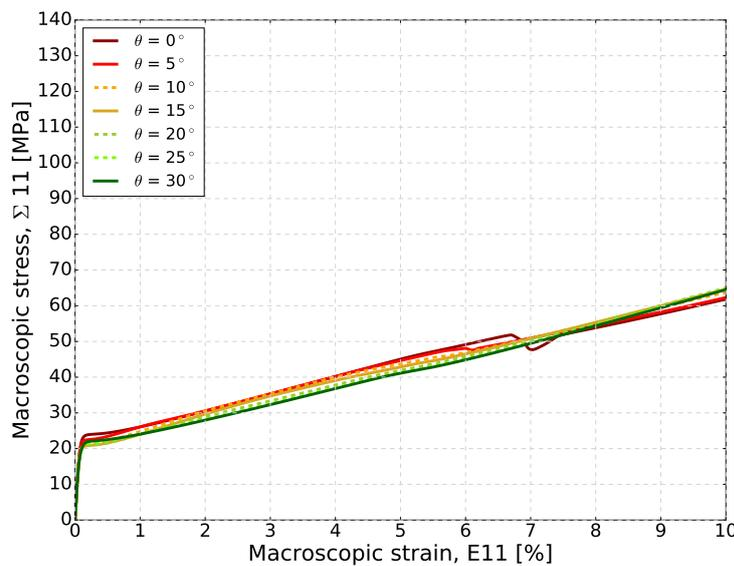
FIGURE 7 – Macroscopic behavior of the hexagonal lattice solicited in all the in-plane directions.
