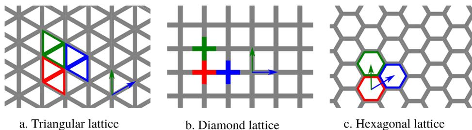
FIGURE 1 – Lattices topologies and their corresponding unit cell employed in FE analyse.
