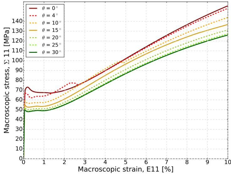
FIGURE 2 – Macroscopic behavior of the triangular lattice in all the in-plane directions.
