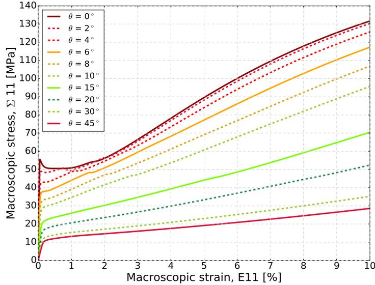
FIGURE 4 – Macroscopic behavior of the diamond lattice solicted in all the in-plane directions.
