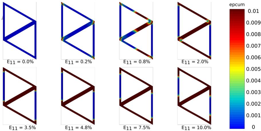
FIGURE 3 – Triangle cell loaded in X direction angle 0
