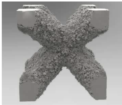
FIGURE 1 – \mu CT Reconstruction - 3\mu\text{m} voxel, scale : 5mm unit cell, 1000\mu\text{m} strut, Adhered particles : 10\text{-}60\mu\text{m}
