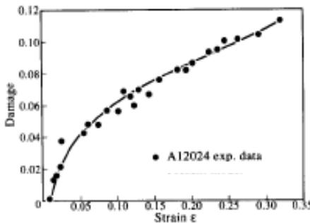
Experimental curve to derive D as a function of p
