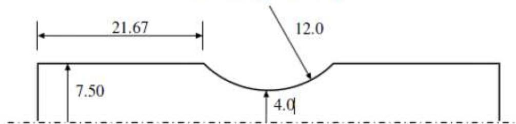
(b) Round bar of the notch radius  $R = 12$  mm.
