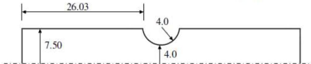
(c) Round bar of the notch radius  $R = 4$  mm.
