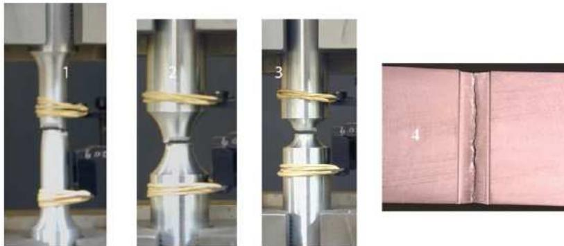
Fracture tests using various sample geometries and testing configuration: Tension, compression, shear
